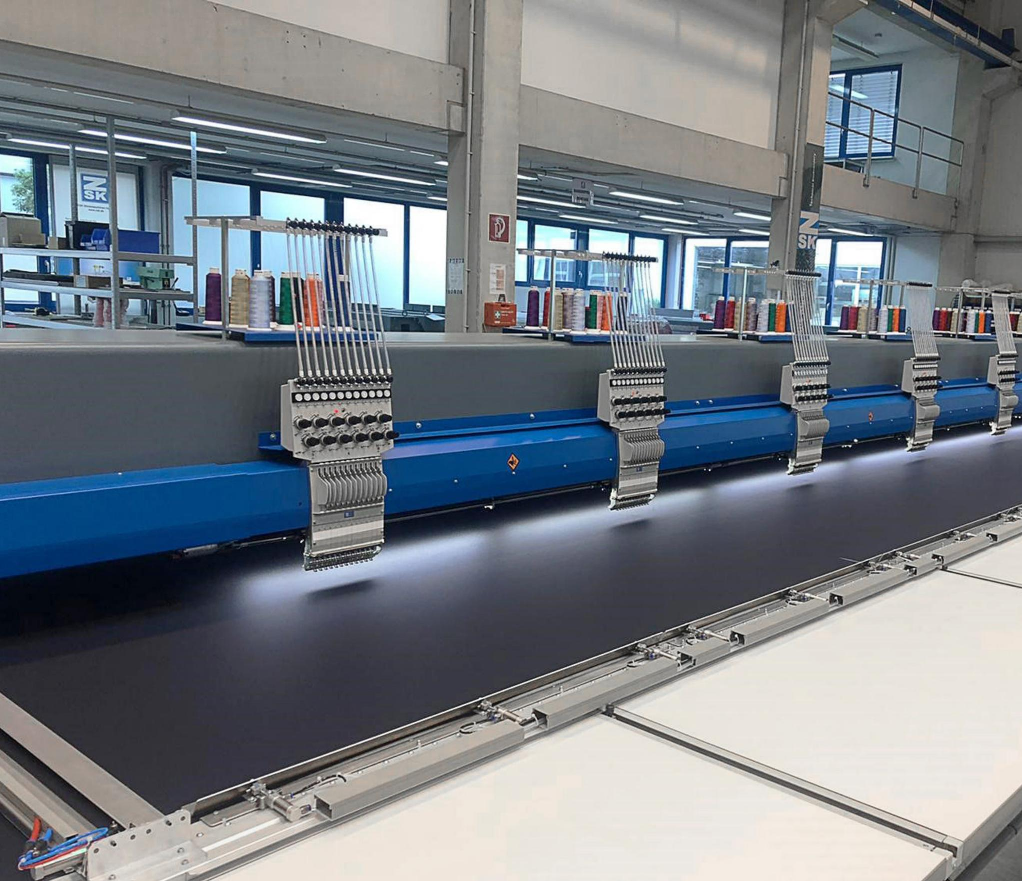
**Pneumatic clamping frame with adjustable depth**
