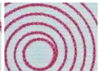
Thread tension: 200 gf
