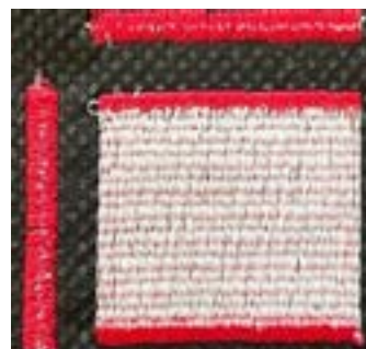
Bobbin thread too tight or upper thread too loose
