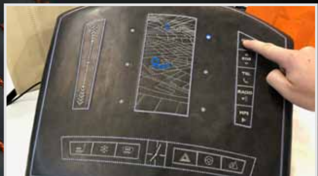
Embroidered Dashboard with Capacitive Sensors
